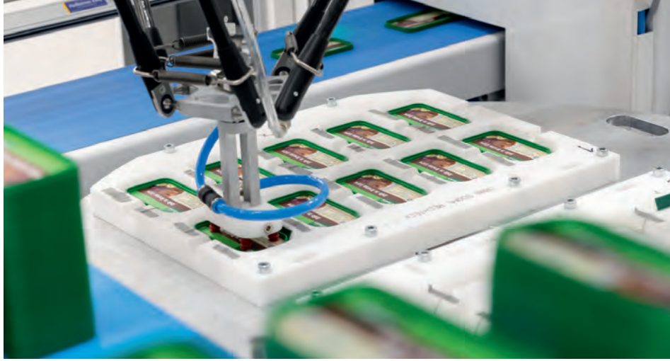
Compressed air serves to transport the parts and eject them from the moulds.
