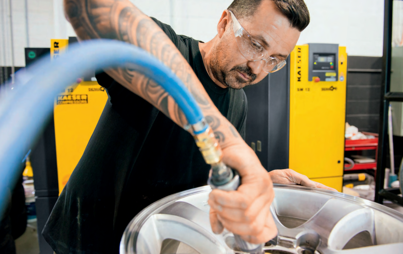
Compressed air is an essential assistant for repair and maintenance tasks; in this case for powering pneumatic tools.
