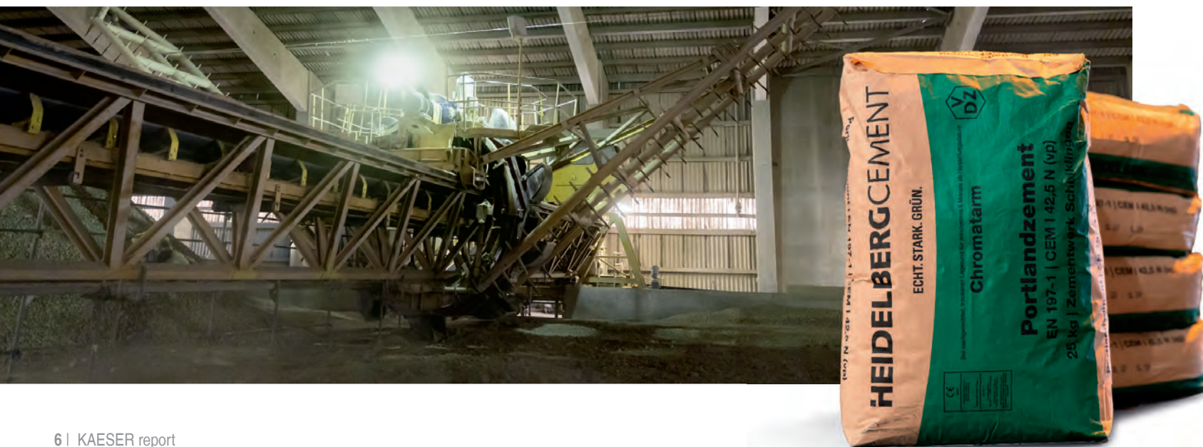
Image left: The raw stone storage area with the conveyor system for transportation of the stone to the mills.
