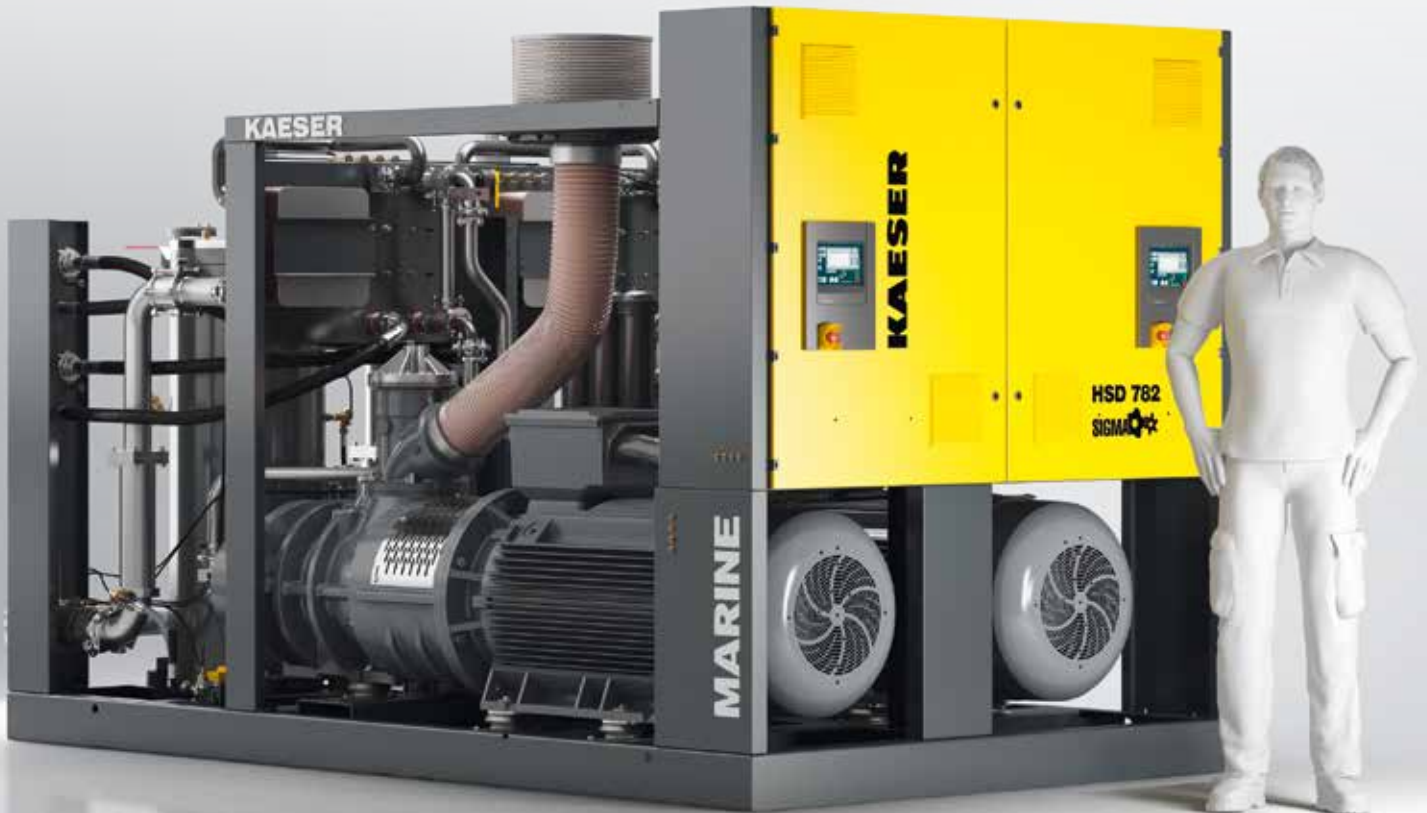
Image: HSD 782 Motor power: 360 to 630 kW FAD: 2.590 to 5.110 m³/h Standard pressure: 8 to 14 bar (g)
